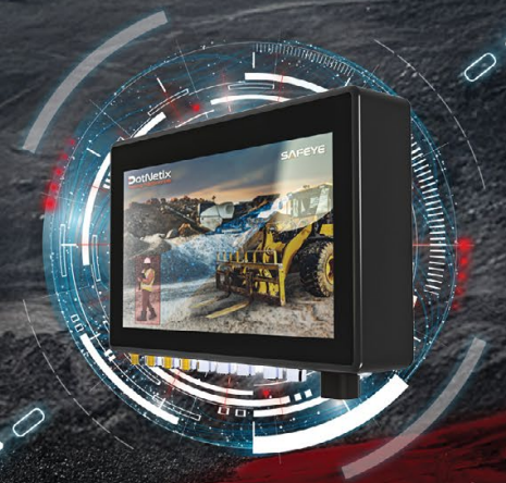
Video display delivers audible and visual warning to operator
